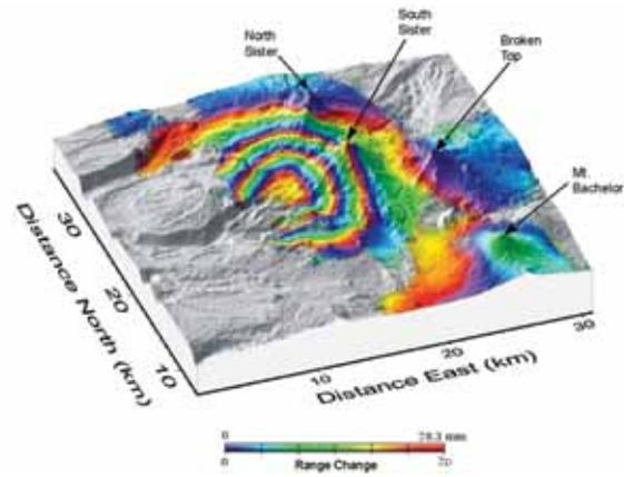
**Figure 3** An area of uplift near the Three Sisters cluster of volcanoes in central Oregon, mapped using satellite interferometric synthetic aperture radar (InSAR). Each concentric circle of red corresponds to approximately 28 millimeters in deformation.
