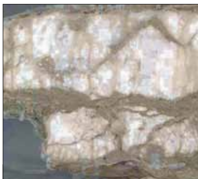
Figure 1. Methane hydrate layered in a one-centimeter thick sample from the Southern Hydrate Ridge, below the seafloor off the U.S. northwest coast.
