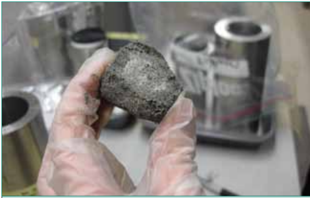
Figure 2. Methane hydrate dispersed through sand deposits from the Alaska North Slope.
